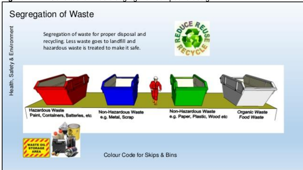
Figure 1 Construction waste segregation compound design
